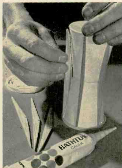
Fig. 7 —Use silastic rubber (or bathtub caulk) to cement paddles to the outside of the drive roller. Be careful not to plug or block the vent holes in paddles.
