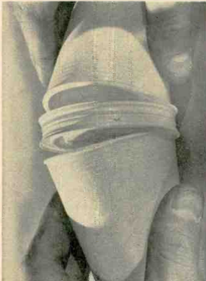
Fig. 3 —The front roller assembly: Glue two Styrofoam cup lids together. Then cut \frac{1}{2} " hole through each lid center for axle. Finally, push cups into lids as shown.
