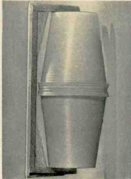
Fig. 4 —Front roller is mounted beneath the movable yoke, using two eyelet bearings and a piece of coathanger wire. Unit functions as the steerable roller axle.
